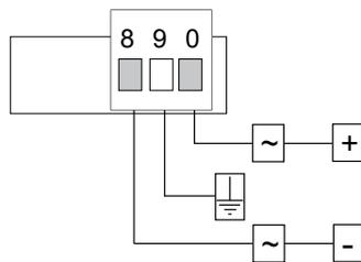
Earth connection - Although a terminal is offered for earth connection, the connection is optional. The instrument does not need this connection for correct functioning nor for compliance with the security regulations.
