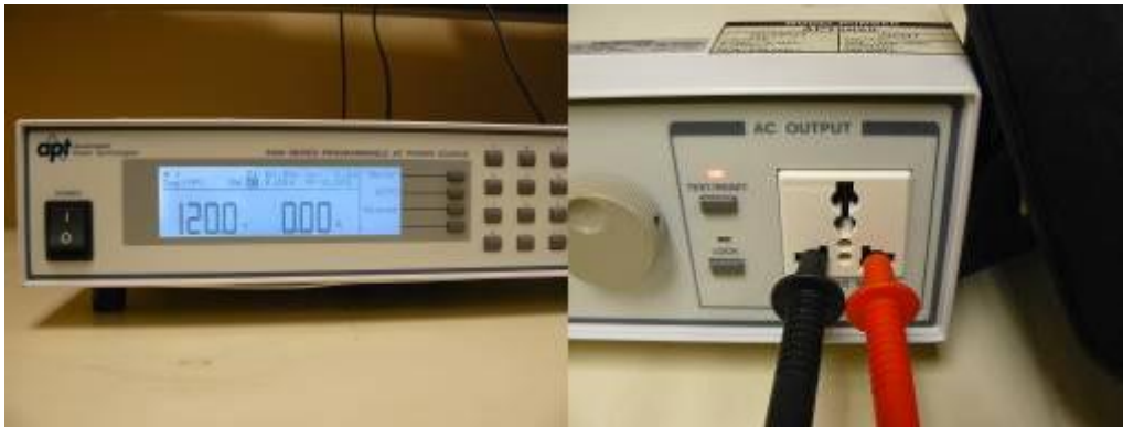
Figure 6a: 6020 source set to 120.0VAC and voltmeter connected between line and neutral output
