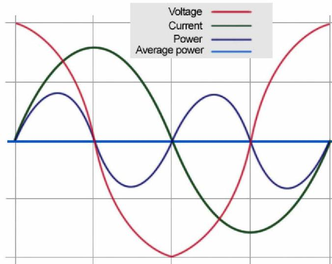
Fig. 5: Voltage, Current and Resulting Power waveforms
