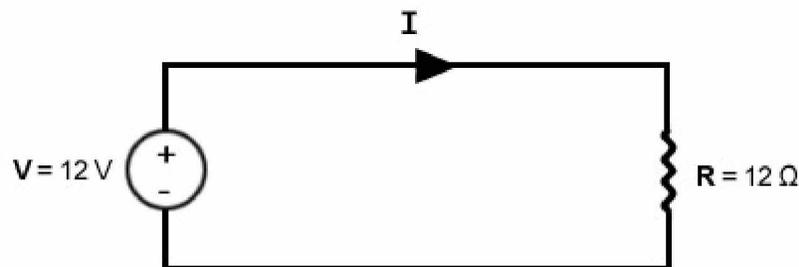
Fig. 3: Simple DC Circuit
