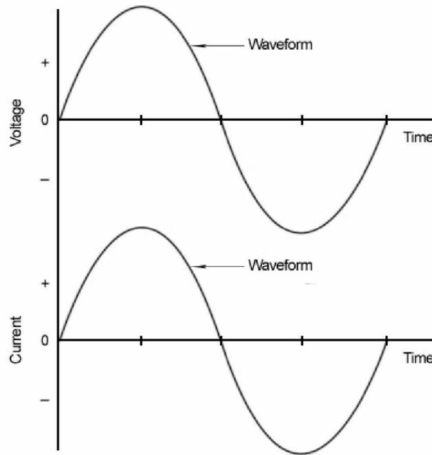
Fig. 4: In Phase Voltage and Current Signals
