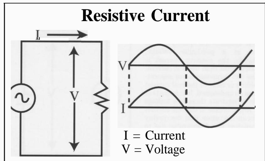
**Leakage current due to the insulation resistance of the product is resistive, and in phase with the applied voltage.**
