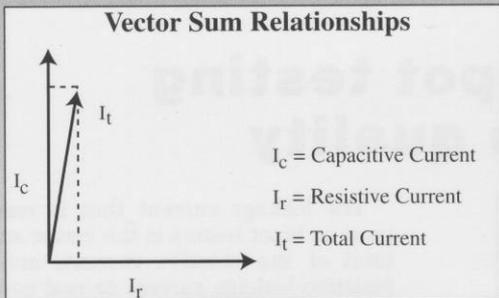
total current sine wave is no longer either in phase or 90 degrees out of phase with the voltage waveform.
