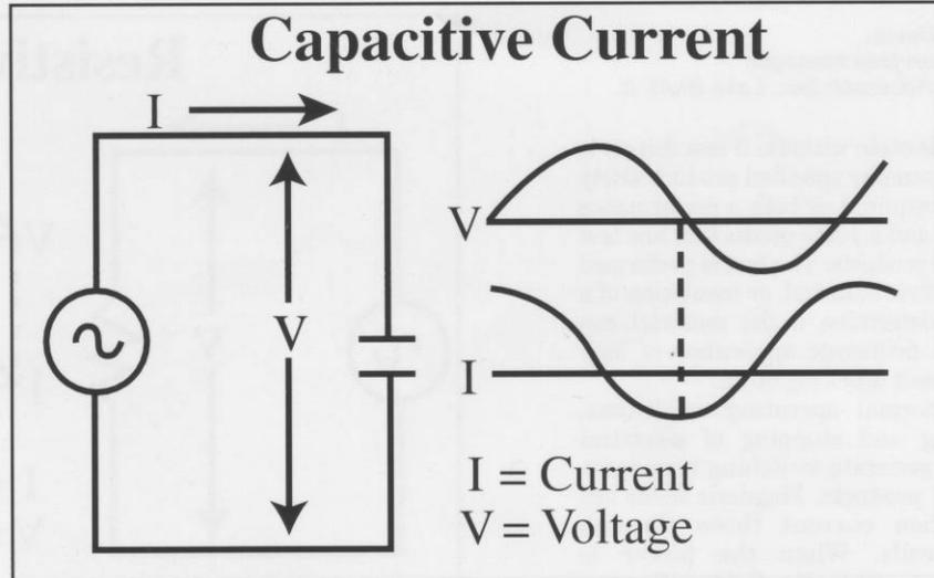
*Application of an ac test voltage to a capacitive element causes a reactive current that is 90-degrees out of phase with the applied voltage.*
