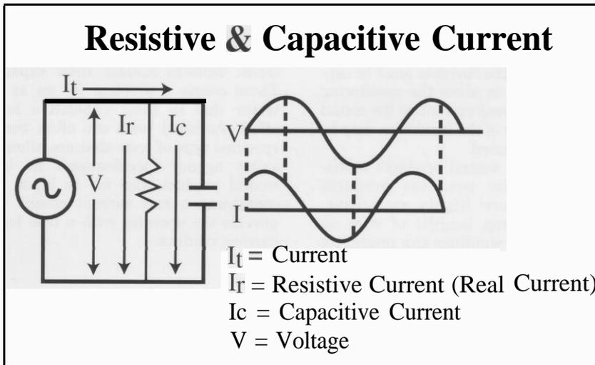
**Real current is due to the insulation resistance of the product and the applied voltage**
