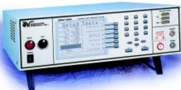
Some of these testers did not shut off the high-voltage circuit when the current trip setting was exceeded. Instead, they incorporated high-reactance transformers, which were current-limited. The voltage collapsed, and the current was limited to a short-circuit current, typically less than 15 mA. Yet these currents are considered dangerous by today's
