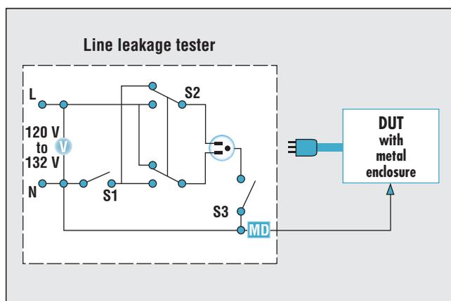
**Figure 3.** The entire enclosure of a Class I product is measured for leakage current.
