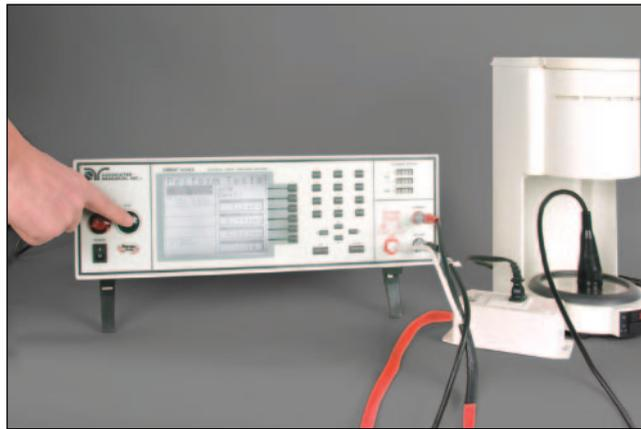
**Figure 1. Multifunction single instrument shown testing a common small appliance.**
