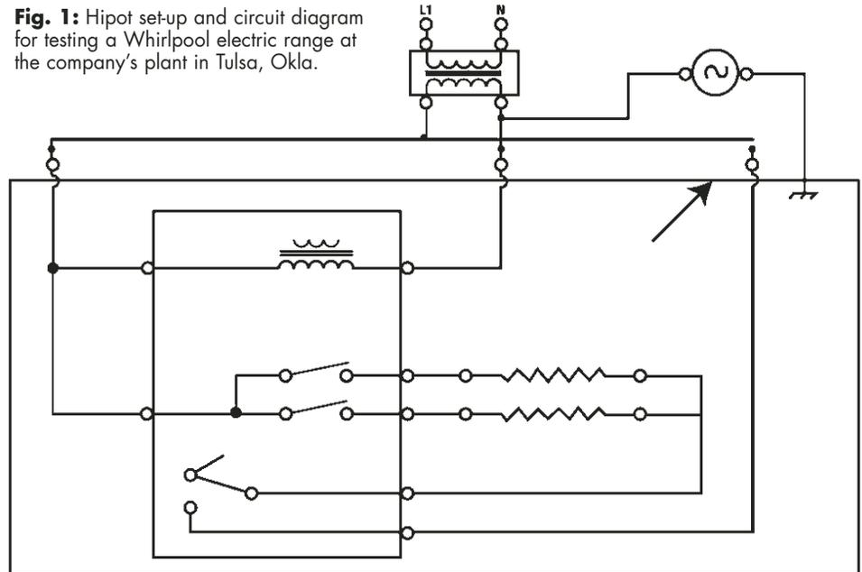
ground, without the isolation transformer, it would see the neutral connection to ground as a fault condition.
