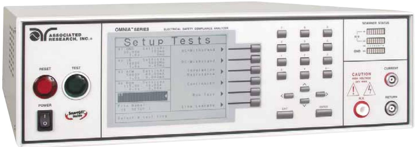
The **OMNIA electrical safety compliance analyzer**, from Associated Research, performs a number of electrical safety tests with a single DUT connection, eliminating the need for the interconnection of multiple instruments. The unit includes AC/DC hipot, insulation resistance, ground bond, line leakage, run tests and optional built-in scanner in a single instrument.
