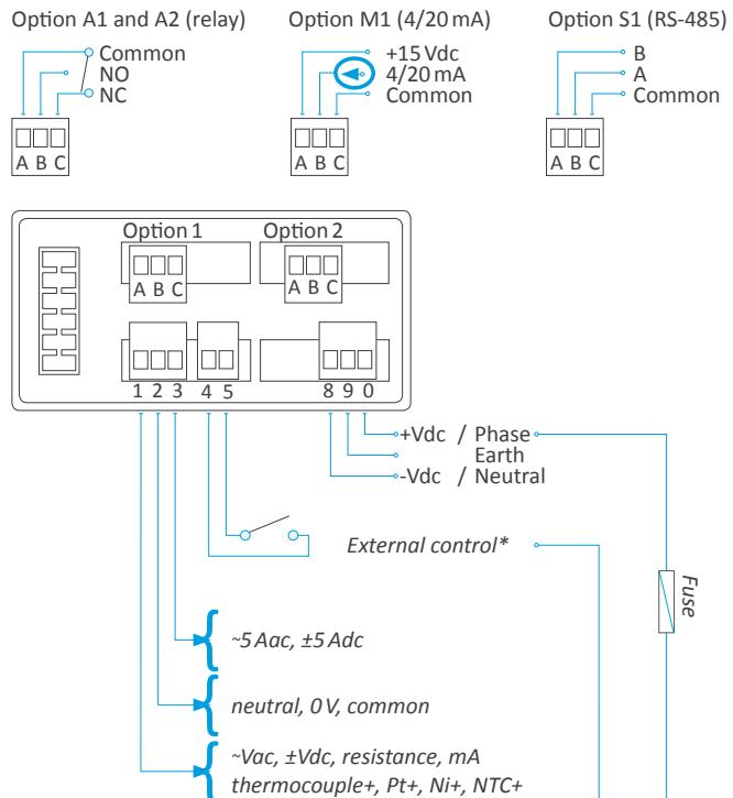
**Warning:** \* Risk of electric shock. Input signal 'terminal 2' is internally connected to external contact 'terminal 5'. When measuring signals with dangerous voltages, apply the appropriate protections to the external contact to isolate the operator from dangerous voltages.
