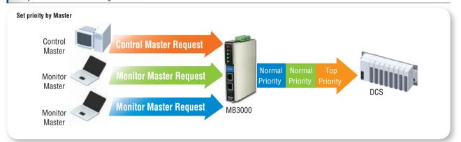
Multiple masters may exist on both the TCP and RTU/ASCII network.
