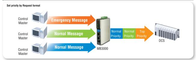
Certain control requests may be sent from many masters, with only one specific request format requiring real-time control (e.g., "turn-off"). Priority control allows a specific request format to be designated
